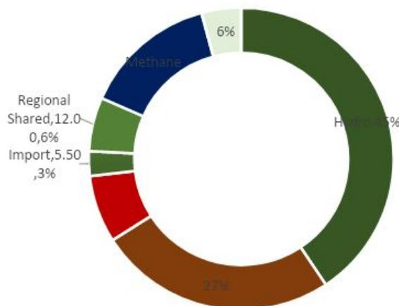
The primary sources of electricity in Rwanda are hydro-power, methane gas, peat, diesel, solar PV, regionally shared hydro-power plants and imports. The total installed electricity generation capacity is on the rise, increasing from 160 MW in 2015 to 218 MW in 2017<sup>5</sup>.
